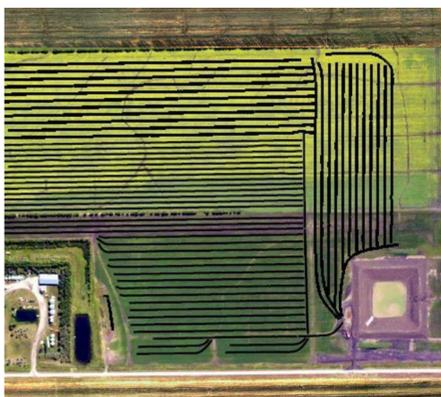
Figure 1. Layout of the study field. Black lines represent the lateral tiles.
