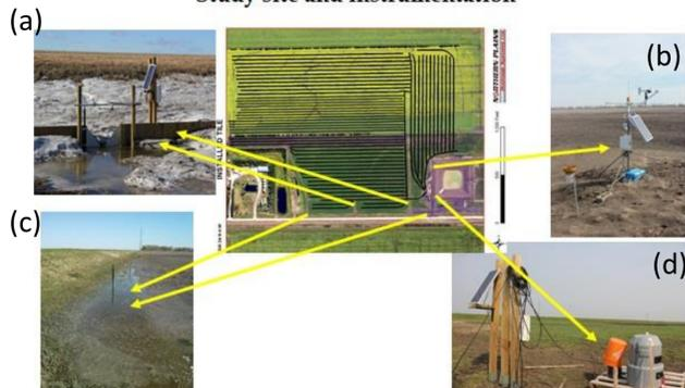
Figure 1. Study site and instrumentation. a. Overland flow monitoring station b. weather station c. ditch monitors d. tile flow monitoring station
